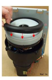
Assemble the top of the fan housing onto the bottom part by tightening the four screws – being careful not to overtighten. Fix angle bracket to base plate (cf. photo ref. 15B).
